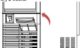
A Note: Be careful when doing the condenser cleaning as the edges of the fins are sharp.
