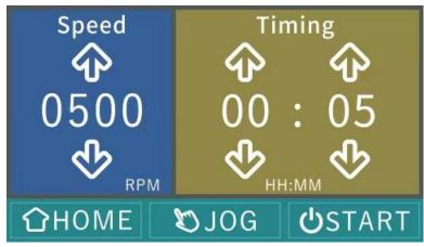
(a) You can adjust the speed by pressing the up and down buttons, and directly press the speed to input it through the keyboard.
