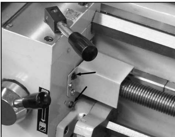
Figure 45: Half-nut gib adjustment location.
