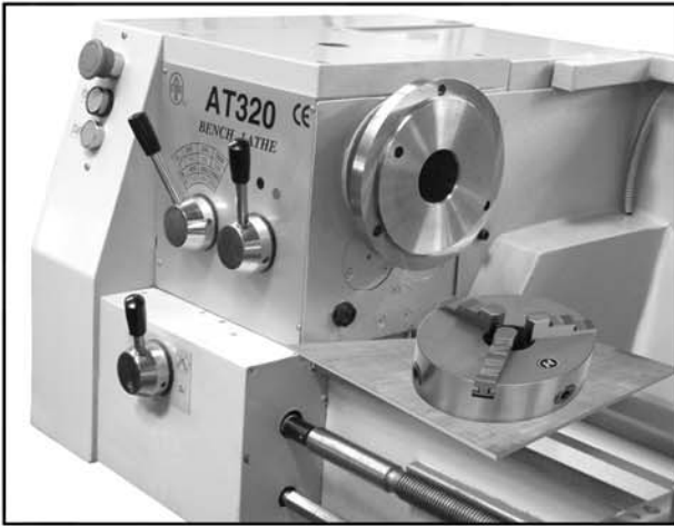
Figure 25: Chuck mounting components.
