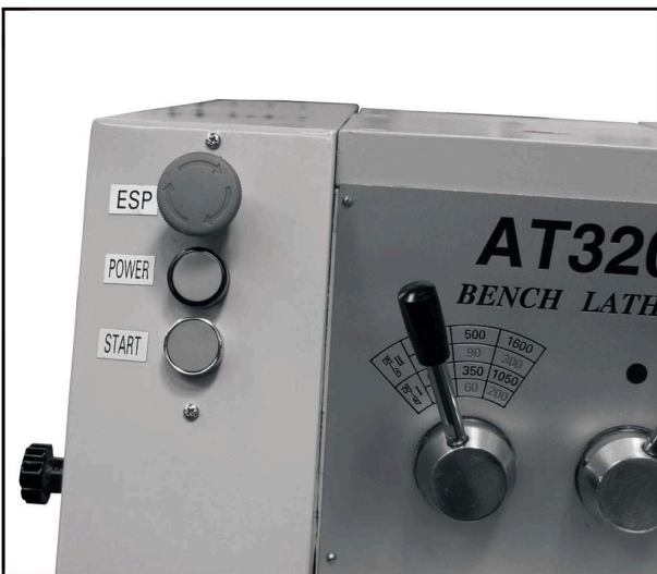
Figure 2: Power lamp and emergency stop location.
