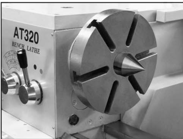
Figure 24: Faceplate and dead center setup.
