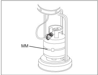
11. Turn the cylinder valve on the tank clockwise to close the propane tank. Attach the regulator (H) to the cylinder valve by turning the regulator coupling nut clockwise. Make sure it is fastened securely and tighten connections by hand only.
