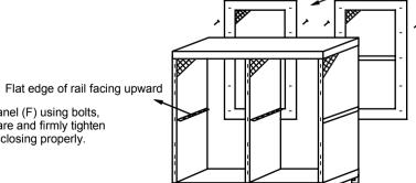
3. Connect the back panels (A) to side panels (E & G) and mid-panel (F) using bolts, washers, and nuts provided (J & K). Ensure the unit remains square and firmly tighten the nuts. Note: out of square assembly will prevent the door from closing properly.
