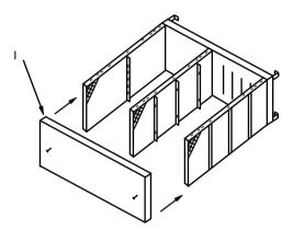
2. Assemble the top panel (I) to the side panels (E & G) and mid-panel (F). Hand-tighten the bolts, washers, and nuts provided (J & K). Ensure the unit is square and firmly tighten the bolts connecting the side and mid panels to the base. Tighten the bolts connecting the side and mid panels to the top panel. Set unit upright.
