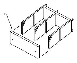
2. Assemble the top panel (G) to the side panels (E) and mid-panel (F). Hand-tighten the bolts, washers, and nuts provided (H & I). Ensure the unit is square and firmly tighten the bolts connecting the side and mid panels to the base. Tighten the bolts connecting the side and mid panels to the top panel. Set unit upright.
