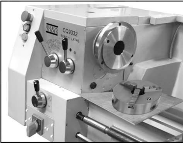
Figure 25: Chuck mounting components.
