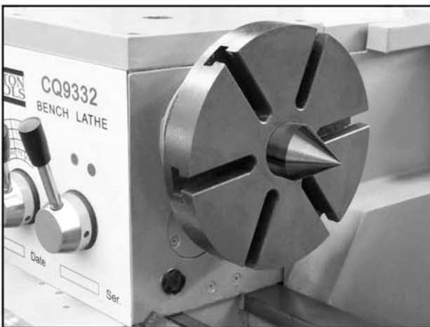
Figure 24: Faceplate and dead center setup.
