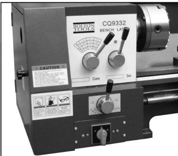
Figure 2: Power switch location.
