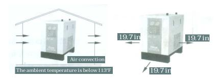
Install in the breezy place, and the ambient temperature can't extend  $45^{\circ}\text{C}.$
