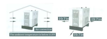
Install in the breezy place, and the ambient temperature can't extend  $45^{\circ}$ C.
