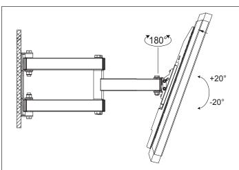
Step-4: Adjust the angle of the panel TV between +20 and -20 degree to a suitable position, and screw up the hook screw at last.
