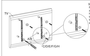
Step-2: Select suitable screws from the screw package according to the size of the holes in the back of TV.Fix the two hanging arms onto the back of TV by screws into the holes.
