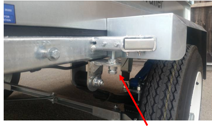
4.4.5 Upper suspension adjusting bolts
