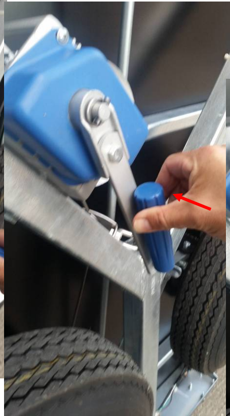
3.2.10 Fold in the winch handle
