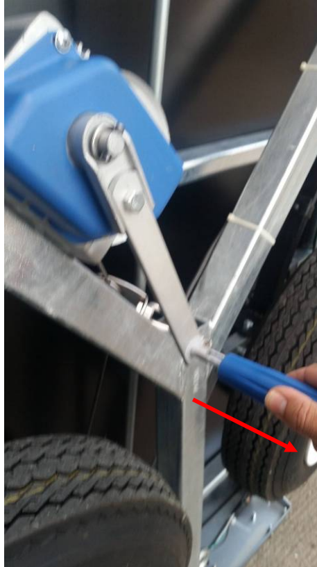
3.2.10 Fold in the winch handle
