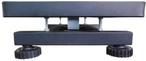
For preventing the loadcell from being damaged during transportation, there are four protection screws in the middle of the scale, please adjust the four screws before using after receiving the goods, or the scacle can't be used for weighing.
