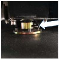
Remove Hexagon Screw 1 from motor shaft
