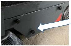
Unscrew the 3 hand screw screws on the lower guard plate
