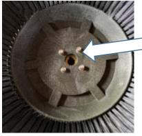
Open the sweeper and brush the 4 hands under the screw screws
