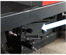
Unscrew the 4 hand screw nuts on the rocking arm and baffle, and remove the rocking arm and baffle
