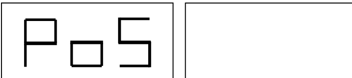
Fig. F3.15 - Balancing planes search: the left display indicates that the sensor is exactly on the internal balancing plane
