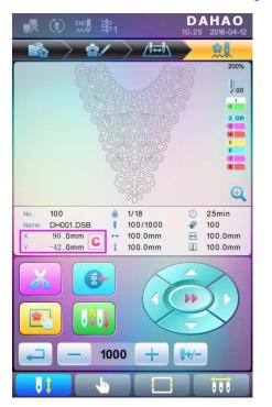
Press " ev, to enter the interface for frame selection and position setting; then press " vey, to enter the interface for setting related parameters, where user can input the coordinates of XY in the main interface.
