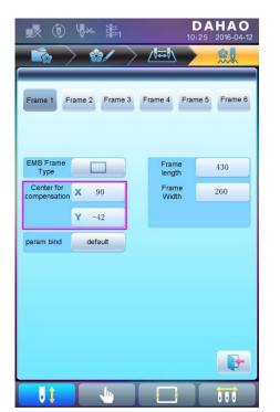
There are four parameters: "X direction center" means the distance at X direction between the frame center and X- direction position limitation optical coupler; "Y direction center" means the distance at Y direction between the frame center and Y+ direction position limitation optical coupler. "X direction frame size" means the embroidery range of the frame at X direction; "Y direction frame size" means the embroidery range of the frame at Y direction.
