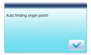
System will move the frame automatically and determine the origin according to the limit switch. So please ensure that the limit switch has been installed into the machine and activated.
