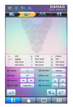
System will display independently the modification windows for X Scale and Y Scale for users to set respectively.
