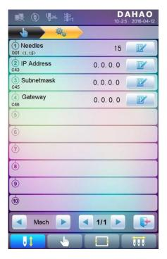
2. Press the parameter to be set and input the new value by the number keys.
