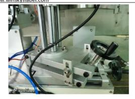
Angle adjustment base: If the one label end is higher or lower than another ending when labeling, then need to loosen the screw and turn the handwheel to adjust until the label two ends are in same level, then tighten the screw
