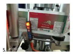
Label sensor setting: if sensor can't detect label and here is the re-setting way.
