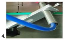
Fiber sensor: The detection position can be adjusted appropriately according to the principle of labeling immediately when the fiber sensor detects the product
