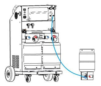
Through tank fittings, connect either HP or LP hose with external refrigerant R134a or
