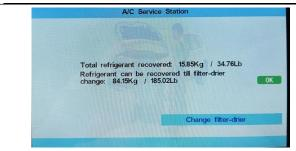
When machine is switched on, filter-drier life is displayed. Click OK to enter main menu.
