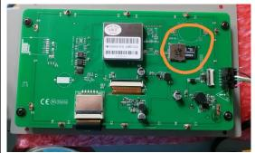
Swith off the machine, remove the SD card and restore the machine:
