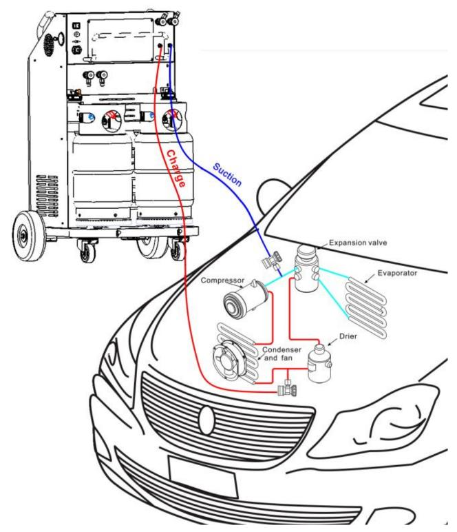
Warning: Except the situations clearly stated in the manual, during all equipment operations, please maintain the vehicle engine and A/C off, otherwise unexpected damages may be caused.
