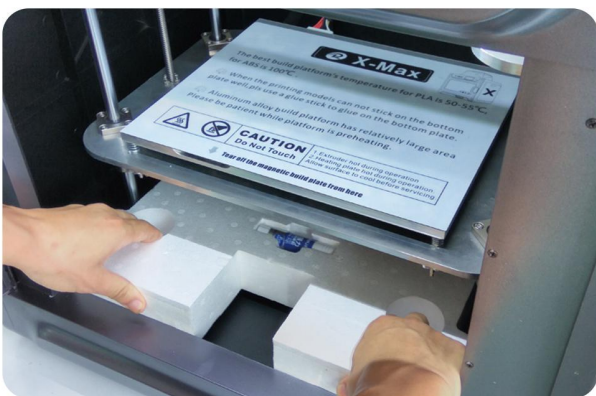
17. When build platform up to the middle, take out the foam from the bottom of build bed.
