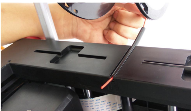
7. Insert the filament into the filament guide.
