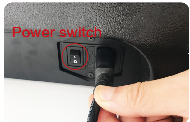
12. Plug in the power cord at the back of the 3d printer's lower right corner, then turn on the power.
