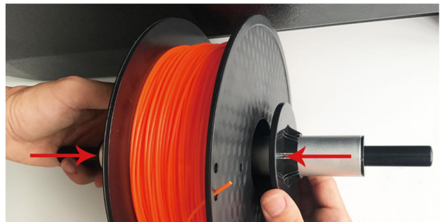
4. Put the gasket left and right to fix the filament.
