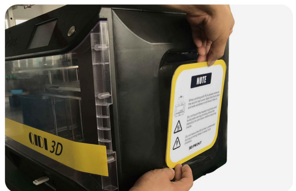
12. Install the magnetic side window.
