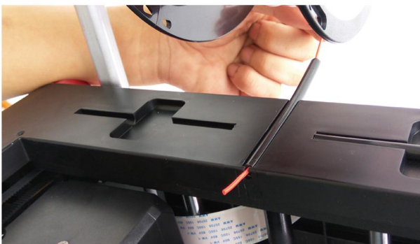
7. Insert the filament into the filament guide.
