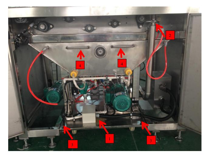
$\bigcirc$  The slurry tank can be pulled out for cleaning. The removal sequence for the tank is:
