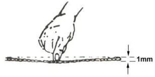
Figure (1) Adjusting Blade Tension
