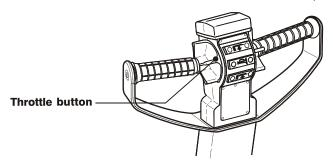
Move the handle all the way down or all the way, up to apply the brake
