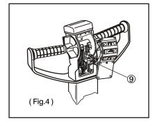
(4) Tighten the 2pieces of fixing bolts #9.(Fig.4)
