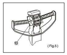
(5) Fix the cover back and tightening the 6 pieces of bolts. (Fig. 5)
