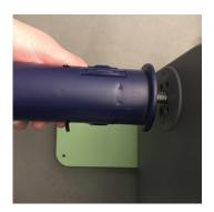
Step 2: Screw the six screwdriver unscrewed at the bottom of the machine. And pull out the support foot of the machine.
