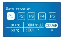
There are 5 cleaning modes (P1, P2, P3, P4, P5) for user. Storage the parameters of Main Interface to P1-P5 so that user can select the parameters directly from P1-P5 for next using.
