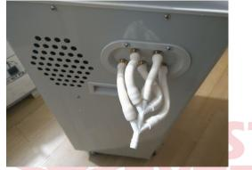
3), Resisted Corrosion: the body of pump is made of high quality plastic, the spare part of it is made of stainless, copper, or plastic parts(PTFE), it is not influenced on acid base, other corrosive matter, etc., do not need to use vacuum oil, it doesn't pollute lab.
