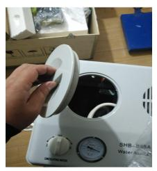
Then infuse water at middle upper position of water level meter, it will be ok for working or circulating water
