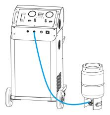
Through tank fittings, connect either HP or LP hose with external refrigerant R134a or HFO-1234yf, and turn on the machine, select corresponding refrigerant type, run recovery to fill R134a or HFO-1234yf tank with refrigerant.
