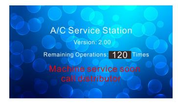
Upon 600 operations having been made, the machine will display the following message while the machine stops working. Service has to be made to reset service interval time again.
