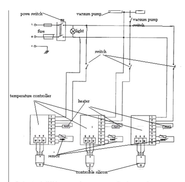
Explanation: 1, 6090 has two set of temperature controllers, heaters, and sensors.
