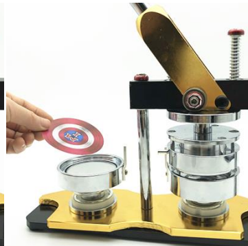
Step 1: place metal tin shell in left mold. Then place circular printing paper on metal tin shell.
