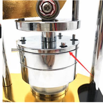
Step 4: rotating the machine, press down the handle. There must be no gap in the top die when press the right mold.
