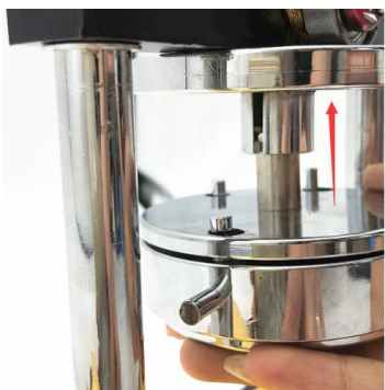
Step 1: set into upper mold. Align the bump with the groove.
