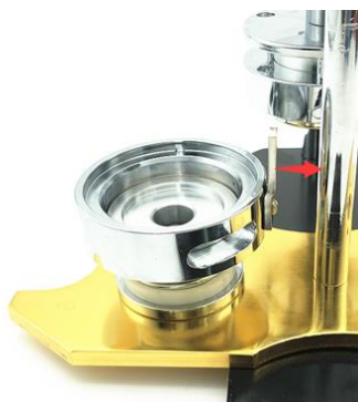
Step 2: put right mold on the B plate. Make sure the baffle align to the column.
