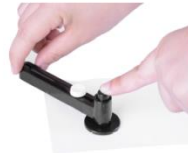
Step 4: rotating the machine, press down the handle. There must be no gap in the top die when press the right mold.
