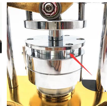
Step 3: press down the handle. Make sure there will be some gap in the top die when you press the left mold.
