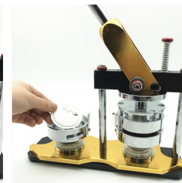
Step 2: place plastic film on circular printing paper. Then rotating the machine, place plastic pin badge on right mold.
