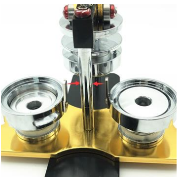
Step 3: put left mold on the other plate. Make sure the two baffles align to the column.
