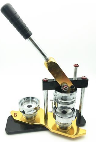
Step 3: put left mold on the other plate. Make sure the two baffles align to the column.
