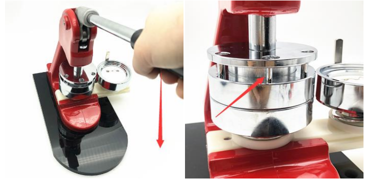
Step 3: press down the handle. Make sure there will be some gap in the upper mold when you press the left mold.
