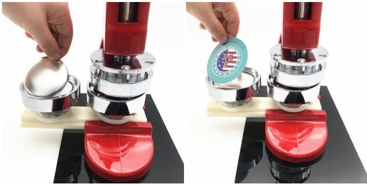
Step 1: place metal tin shell in left mold. Then place circular printing paper on metal tin shell. The paper size should be the same size to the plastic film.
