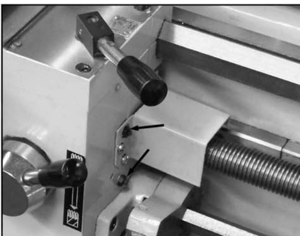
Figure 38: Half-nut gib adjustment location.
