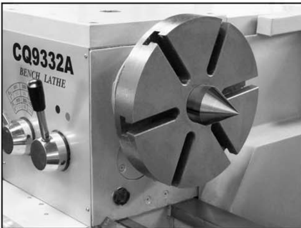
Figure 24: Faceplate and dead center setup.
