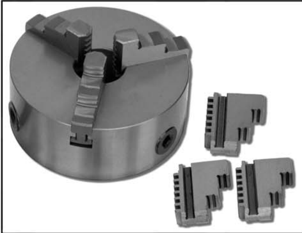
Figure 27: Chuck and jaw selection.
