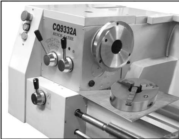
Figure 25: Chuck mounting components.
