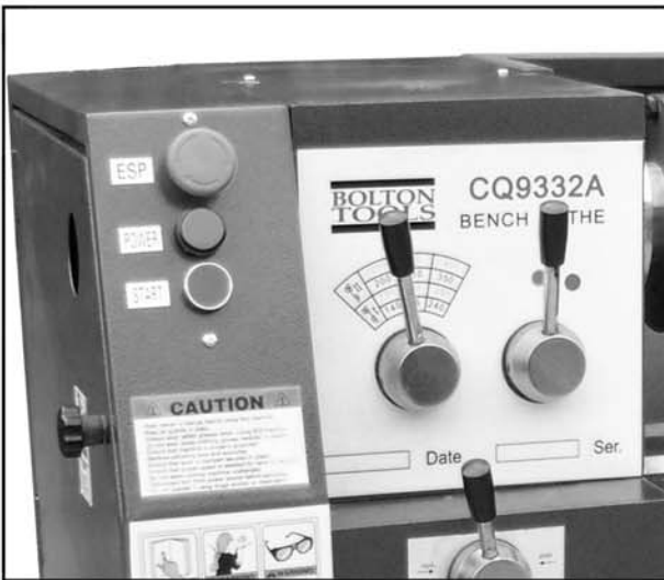
Figure 2: Power lamp and emergency stop location.
