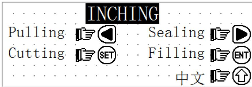
The meaning of INCHING is that we can make the bag by hand manually.
