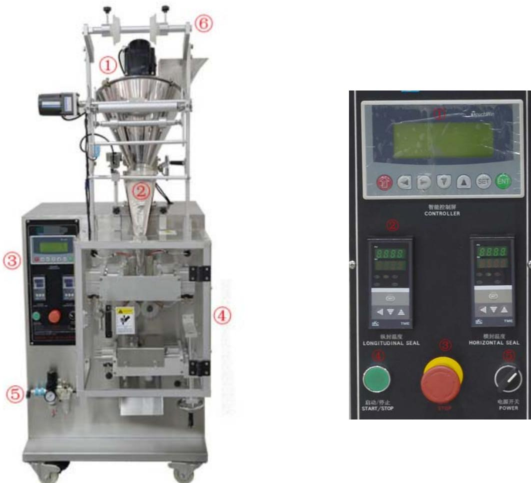
①Auger filler and Hopper-Measuring and Filling Function
