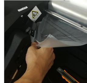
**Step 5: Press “In/Out” and pull the film slightly at the same time.**
